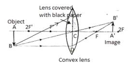
In the second case the upper half of the lens is covered with black paper. Light rays coming from the object are refracted only from the lower half and the image is formed, whereas in the upper half the light rays are blocked.
