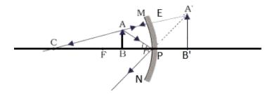
A virtual, erect and magnified image is formed.
