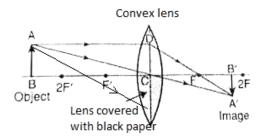
In the first case the lower half of the lens is covered with black paper. Light rays coming from the object are refracted only from the upper half and the image is formed, whereas in the lower half the light rays are blocked.
