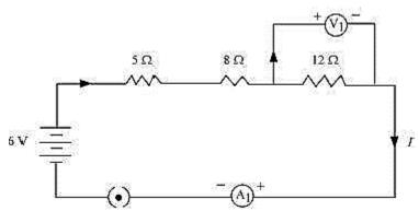
Given three resistors  $R_1 = 5\Omega$ ,  $R_2 = 8\Omega$ ,  $R_3 = 12\Omega$  are connected in series. And V be the potential across the circuit and  $V_1$  be the potential difference across  $R_1 = 5\Omega$ ,  $V_2$  be the potential difference across  $R_2 = 8\Omega$ ,  $V_3$  be the potential difference across  $R_3 = 12\Omega$ .
