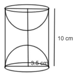
The total surface area of the article = CSA of cylindrical part + 2CSA of hemispherical part
