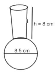
Volume of the vessel = Volume of sphere + Volume of cylinder
