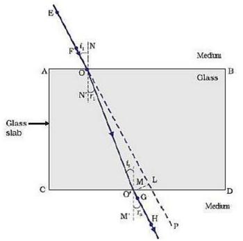
EF is the incident ray and GH is the emergent ray which is parallel to the incident ray. Marks: 2
