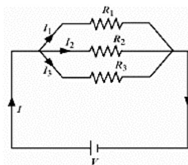
The given figure shows a circuit consisting of three resistors  $R_1$ ,  $R_2$  and  $R_3$  connected in parallel. The total current in the circuit ( $I$ ) gets divided among the three resistors as  $I_1$ ,  $I_2$  and  $I_3$ .
