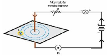
The concentric circles represent the magnetic field lines around the current carrying conductor (copper wire).
