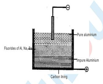
On passing electric current, aluminium ions from the middle layer are discharged at the cathode. An equivalent amount of aluminium goes into the middle layer from the bottom layer. The impurities are left behind. Oxygen is liberated at the anode. Oxygen reacts with the carbon anode. Hence, the anode is gradually consumed.
