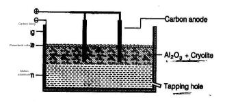
Alumina melts at 200°C. It is a bad conductor of electricity. But when mixed with cryolite and some calcium fluoride, the mixture becomes a good conductor of electricity, and melts at 900-950°C. The iron cell is lined inside with gas carbon which serves as cathode. Carbon rods act as anode. The electrolyte, thus, contains  $Na^+$ ,  $Al^{3+}$ ,  $F^-$  and  $O^{2-}$  ions.
