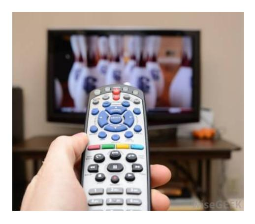
The remote controls used on televisions, VCRs, and stereos all use infrared communication. Many computers and devices have an IrDA port that enables transfer of data using infrared light rays. Transfer rate= 1 Mbps- 4 Mbps. It has wavelength of 700 nm to 1 mm and frequency ranges from 300 GHz to 430 THz.
