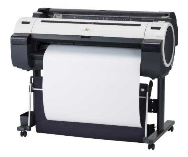
Plotters can automatically change their pens and so can produce colour output. The lines drawn by a plotter are continuous and very accurate. Plotters are very slow but produce high quality output. The quality of the output produced by ink jet printers is now very good and large format (big) ink-jet printers are steadily replacing plotters for most tasks.
