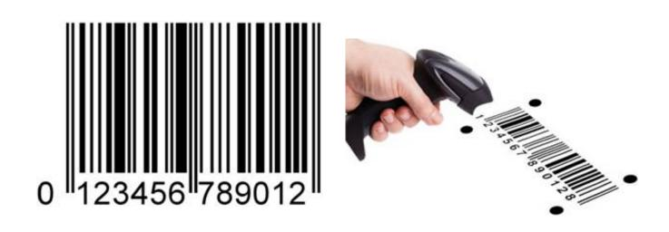
Bar Code Reader scans a bar code image, converts it into an alphanumeric value, which is then fed to the computer to which bar code reader is connected.
