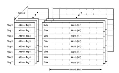
Way 2 Address Tag 2 Valid Words [0-7] Valid Address Tag 3 Way 3 Words [0-7] Address Tag 4 Valid Words [0-7] Way 4 Valid Way 5 Address Tag 5 Words [0-7] Valid Words [0-7] Way 6 Address Tag 6 Valid Way 7 Address Tag 7 Words [0-7] 8 Words/Block 32-word blocks (5 bits)
