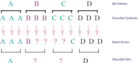
Decoding at the receiver uses a majority logic rule (two out of three wins). If an error occurs the redundancy can help recover the lost information.
