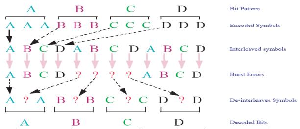
Deinterleaving at the receiver will spread any burst errors that occur during transmission and make it simpler to decode.
