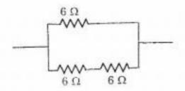
Here, two resistances are connected in series, and this combination is connected to third resistance in parallel to obtain  $4\Omega$  resistance.
