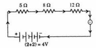
2. Redraw the circuit of Question 1, putting in an ammeter to measure the current through the resistors and a voltmeter to measure the potential difference across the  $12\,\Omega$  resistor. What would be the readings in the ammeter and the voltmeter?
