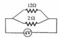
V = 4 V (in parallel V is same for both resistors)
